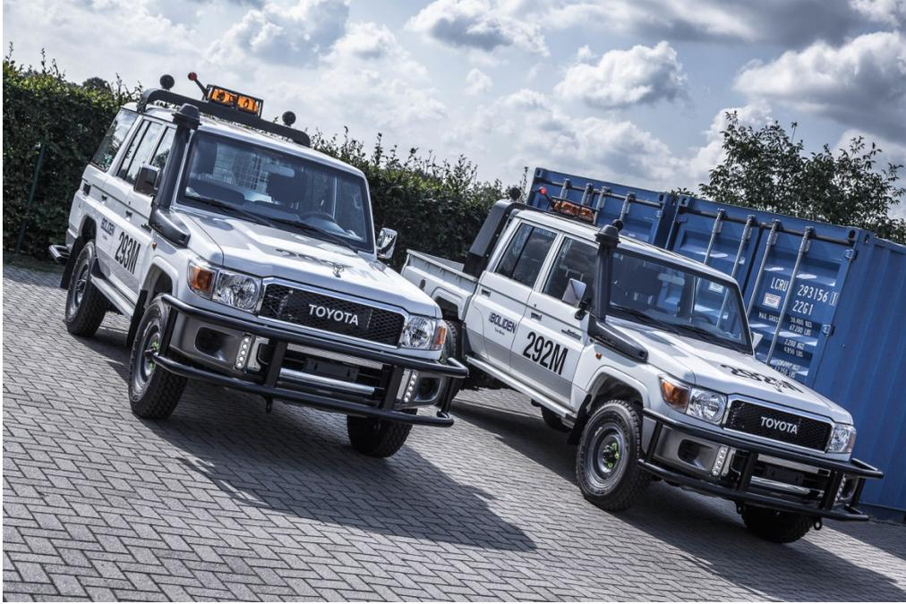
The Toyota Landcruiser 70 Series is the most used light vehicle in mining. The heavy duty frame and powertrain have proven to survive the longest in these rough environments and the basic design makes the Landcruiser the ideal base for special build conversions needed for the different trades inside the mines.
