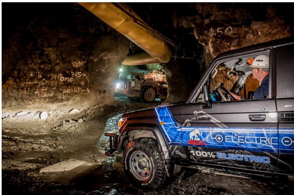
The Tembo 4x4 e-LV electrical Landcruiser is very capable and the standard 28-37kWh battery pack offers 80-100km range, depending on the required range we can offer less or more battery capacity.
